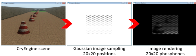
Fig. 2. Image sampling and rendering. The virtual scene (left) was luminance-sampled at 10x10 or 20x20 locations (center) and rendered as corresponding luminance-based phosphene grids (right).
