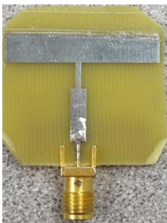
Fig. 3: Microstrip dipole antenna used for testing with phantom material
