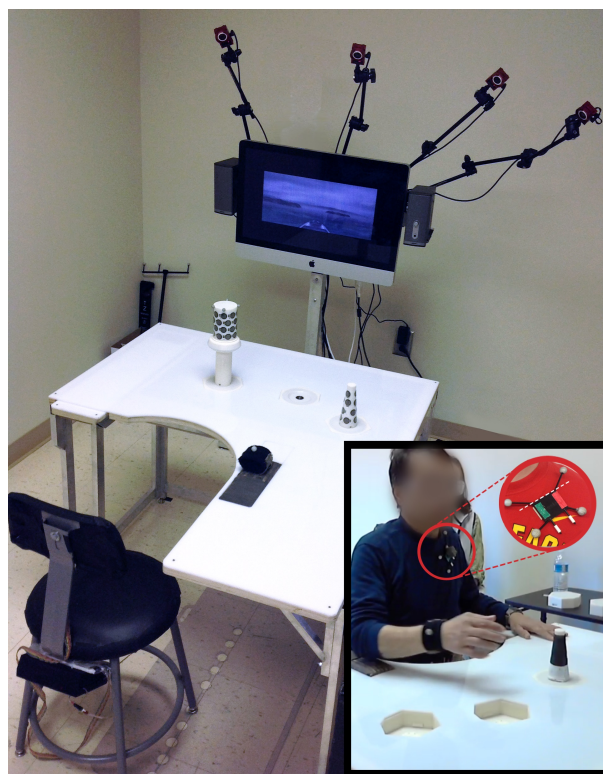
Fig. 1: The HAMRR system used to monitor wrist and torso movements of a stroke survivor during rehabilitation therapy. The system uses four optitrack cameras to track the wrist and torso movements as well as a computer and speakers to provide audio and visual feedback during therapy treatment. In the inset, we see the placement of wrist marker and torso rigid plate (with four reflective markers on the corners) on a participant performing reaching tasks to a cone.
