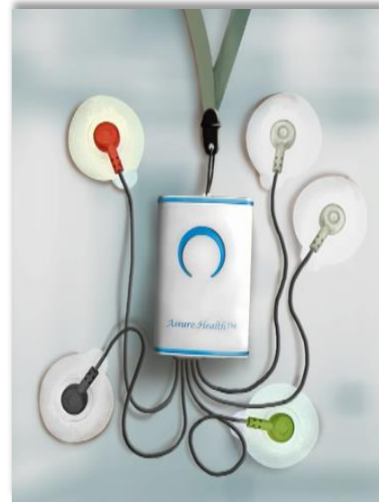
Figure 1. Wipro Assure Health™ ECG necklace with five electrodes to sense three-lead ECG and connects to a smart phone using Bluetooth radio.
