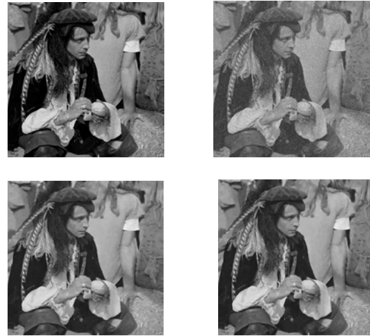
Figure 3. Top left: Original Image, Top right: Noisy image (PSNR=22.11), Bottom left: Denoised image with CSR (PSNR=30.56, SSIM=0.8306) and Bottom right: Denoised image with WCSR (PSNR=30.67, SSIM=0.8361)
