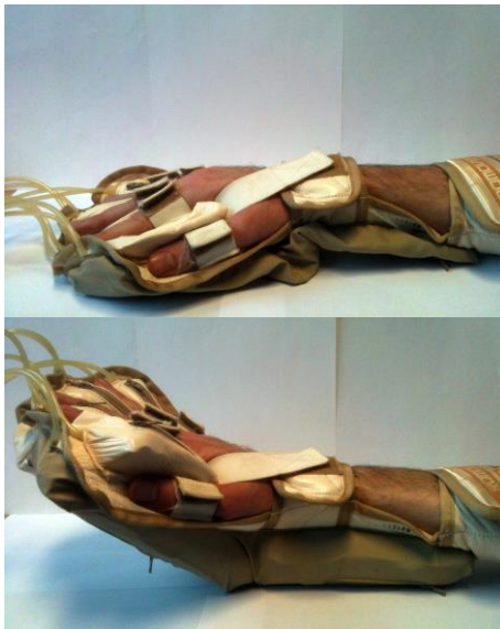
Figure 1. Glove at minimal inflation (top) and at full inflation (bottom)
