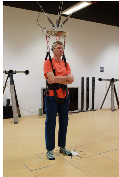
Fig. 1. Subject attached to the FLOAT, standing on force plates
