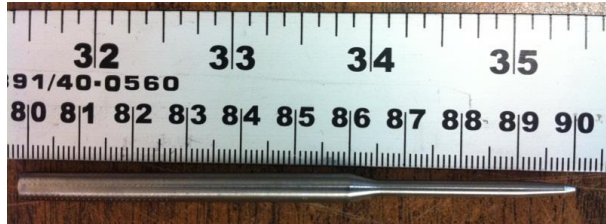
Figure 1. Custom-made indenter used to measure the maximum indentation force.
