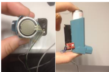
Figure 1. (Left) Top-down view of the recording rig showing FSR on canister. (Right) Side view of recording rig showing microphone placement.
