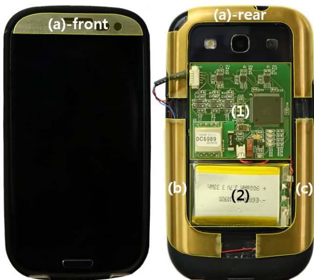
Figure 1. The design of the smartphone-case sensor. (a)-(c) is the metal-based dry electrodes placed in a smartphone case. (1) The multi-channel ECG sensor module with microcontroller and Bluetooth. (2) Li-Polymer battery
