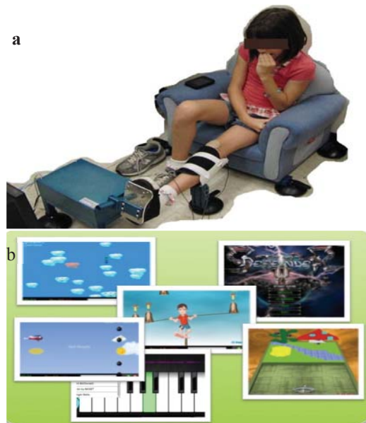
Figure 2. (a) Experimental setup using the portable rehabilitation robot. The affected limb is at full extension and the ankle center of rotation is lined up with the rotation axis of the motor. (b) Screenshots of biofeedback active movement training games.
