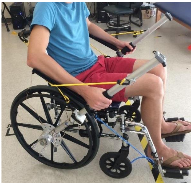
Figure 1. The prototype bimanual LARA wheelchair features two identical levers, with arm support harnesses, coupled to the wheel of the chair with a one-way clutch and to the frame of the chair with elastic bands. This creates a resonant system to assist the user in propelling the chair forward.
