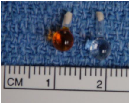
Figure 3. Microsphere bulbs filled with dyed and clear solutions.
