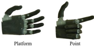
Fig. 2. Grasps and postures provided by the VMG prosthesis.
