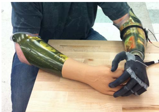
Fig. 4. Transradial bilateral amputee wearing the Vanderbilt Multigrasp Myoelectric Hand (left arm). EMG electrodes are located under the prosthetic socket.
