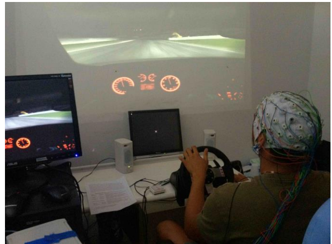
Figure 1. Experimental design employed. The pilot drives the simulated car on a circuit that was identical for all the subjects. Five different experimental conditions have been set up for increase progressively the cerebral workload. This was obtained by performing additional tasks beside the car guide as required by the task of Attention and Vigilance (TAV). TAV tasks are proposed to the subjects on the small monitor just below the track images on the wall and by the acoustic stimulations.
