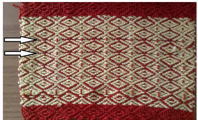
Fig. 5. LCXs (arrowed) weaved into the threads of a textile fabric.
