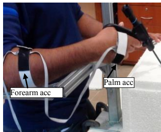
Figure 3. Accelerometer placement on palm and forearm
