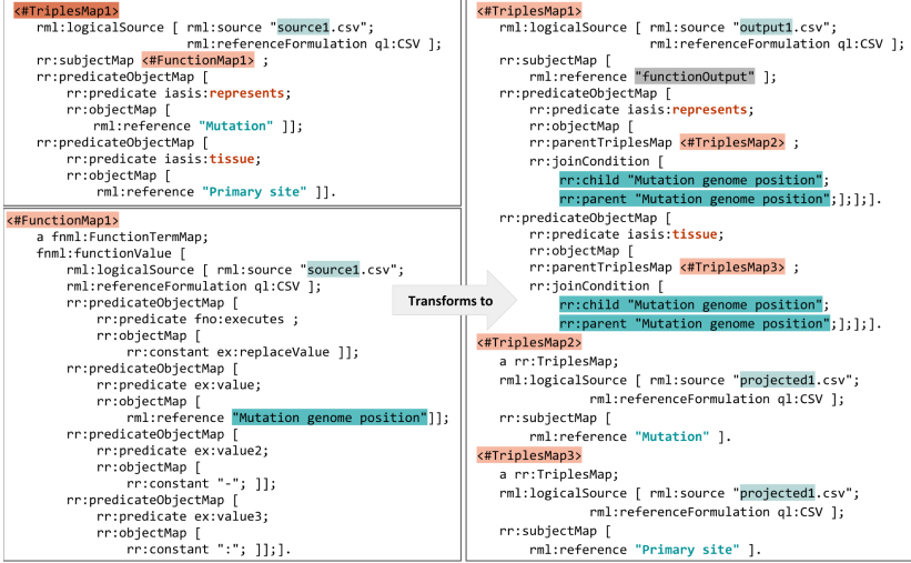
Fig. 6. Example of Subject-based MTR. An example of mappings including a TriplesMaps and FunctionMap are illustrated on the left and their transformed version including three TriplesMap are shown on the right side.
